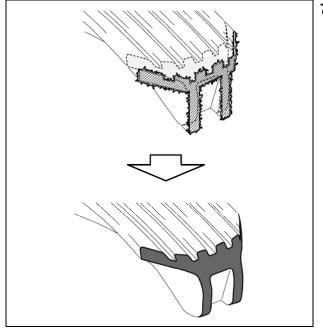
b) Using a reciprocating saw, cut the corners of the pedal.
