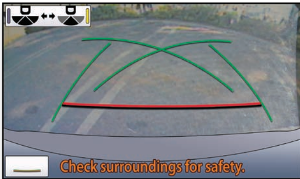
Figure 2 Parking Guide Line Mode
