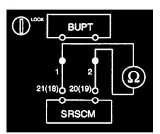
1. Measure resistance between the terminal 1 and 2 of BUPT harness connector.
