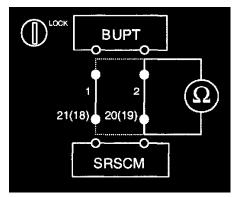
2. Measure resistance between the terminal 2 of BUPT harness connector and the terminal 20(19) of SRSCM harness connector.
