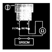
2. Measure resistance between the terminal 21 (18) and 20(19) of SRSCM harness connector.
